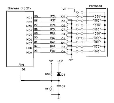
Figure 2-19. Printhead Driver Circuit Diagram
