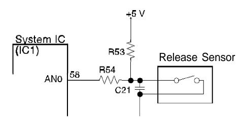
Figure 2-16. Release Lever Position Sensor Circuit Diagram
