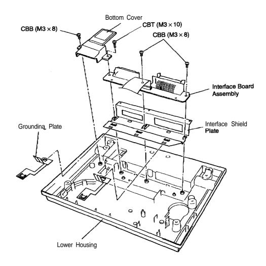
Figure 3-18. Removing the Interface Board Assembly
