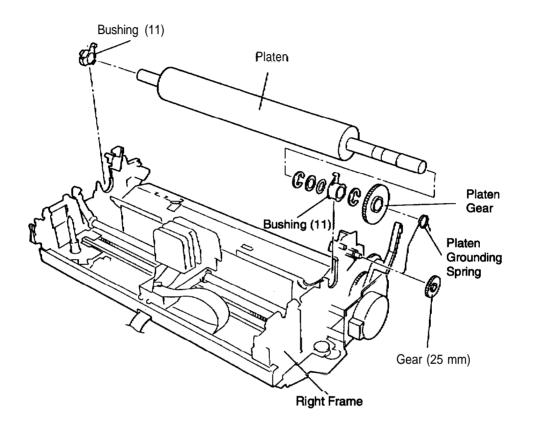
Figure 3-11. Removing the Platen
