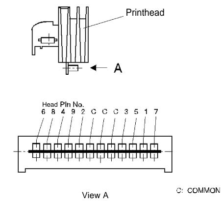
Figure 5-1. Printhead Connector Pin Alignment
