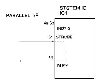
Figure 2-20. Parallel Interface Block Diagram
