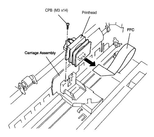
Figure 3-2. Removing the Printhead
