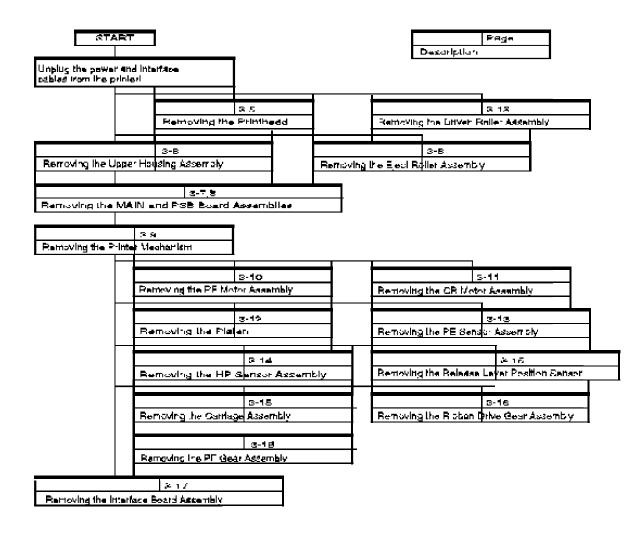
Figure 3-1. Procedure for Disassembling the Printer
