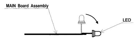
Figure 3-7. Bending the LED Lead Wires
