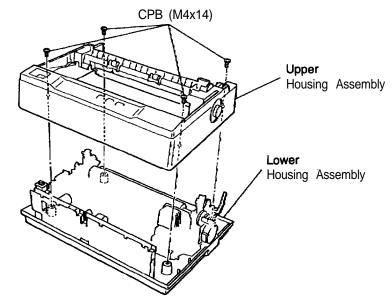
Figure 3-3. Removing the Upper Housing Assembly
