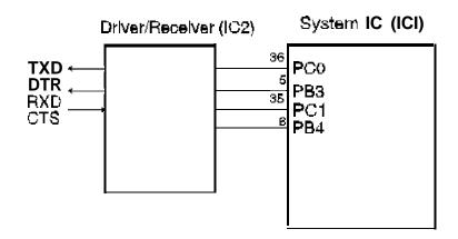
Figure 2-21. Serial Interface Block Diagram
