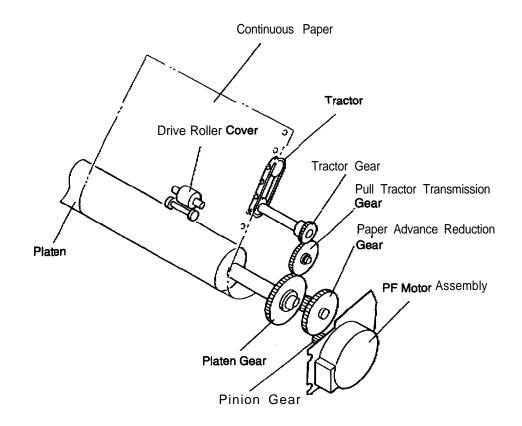
Figure 2-5. Pull Tractor Paper Advance Mechanism
