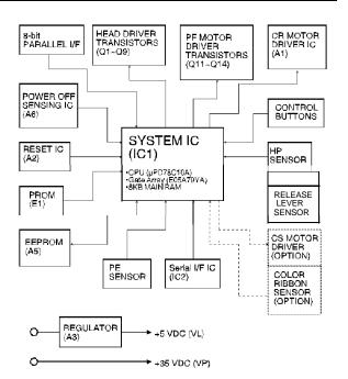
Figure 2-12. Control Circuit Block Diagram
