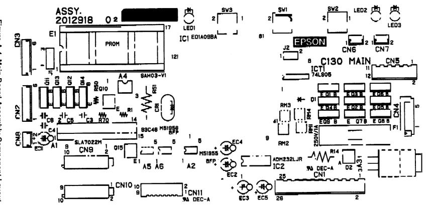
Figure A-4. Main Board Assembly Component Layout
