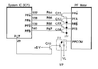
Figure 2-18. Paper Feed Motor Driver Circuit Diagram
