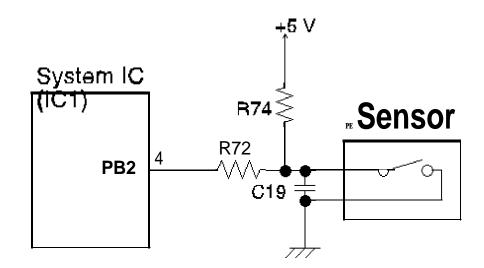
Figure 2-15. Paper End Sensor Circuit Diagram
