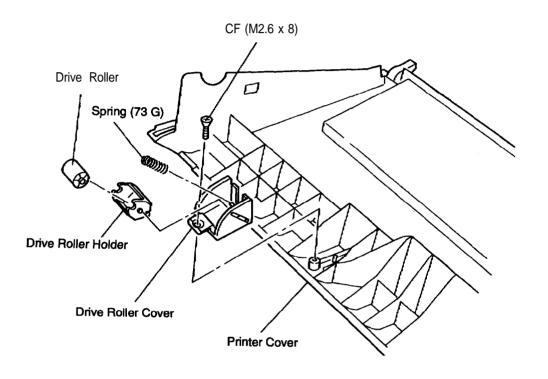
Figure 3-19. Removing the Drive Roller Assembly
