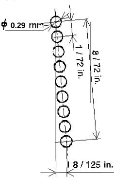
Figure 1-2. Pin Configuration
