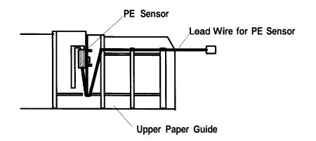
Figure 3-13. Wiring of the PE Sensor
