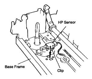
Figure 3-14. Removing the HP Sensor
