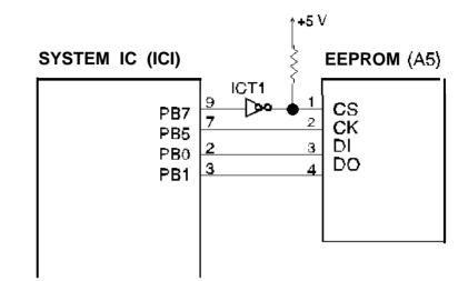
Figure 2-22. EEPROM Control Circuit Diagram
