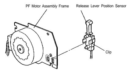
Figure 3-15. Removing the Release Lever Position Sensor
