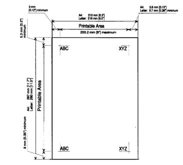
Figure 1-3. Printable Area for Cut Sheets Using the CSF
