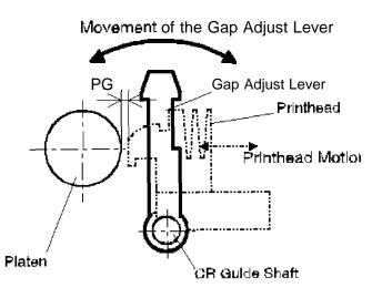
Figure 2-10. Platen Gap Adjustment Mechanism
