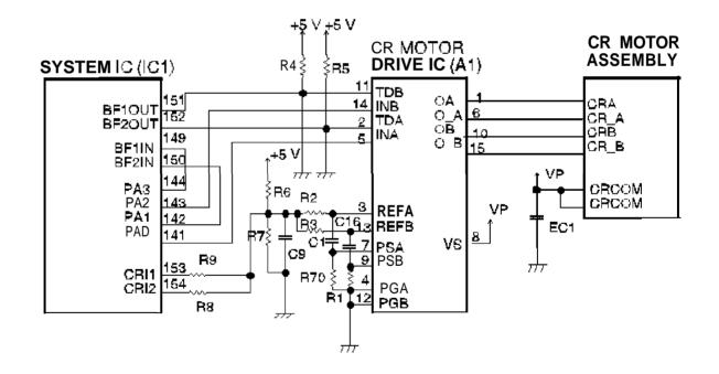
Figure 2-17. Carriage Motor Driver Circuit
