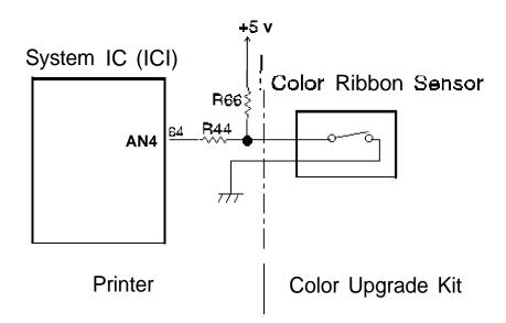
Figure 2-24. Color Ribbon Sensor Circuit Diagram
