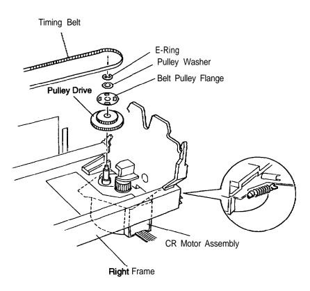
Figure 3-10. Removing the CR Motor Assembly
