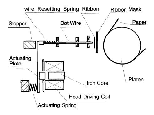
Figure 2-1. Printhead Operation Principles
