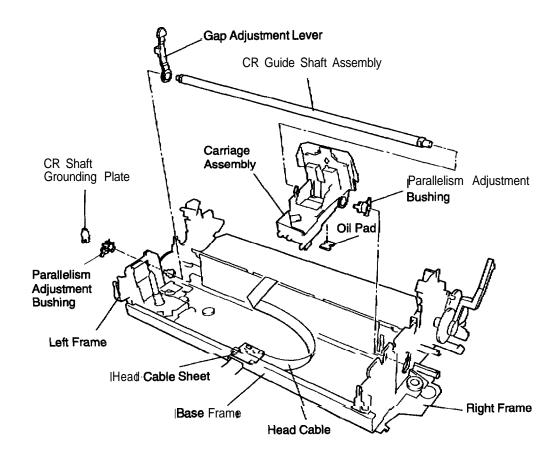
Figure 3-18. Removing the Carriage Assembly
