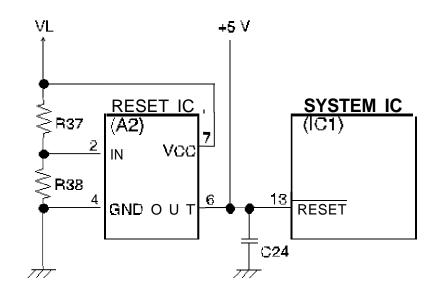
Figure 2-13. Power On Rest Circuit Diagram
