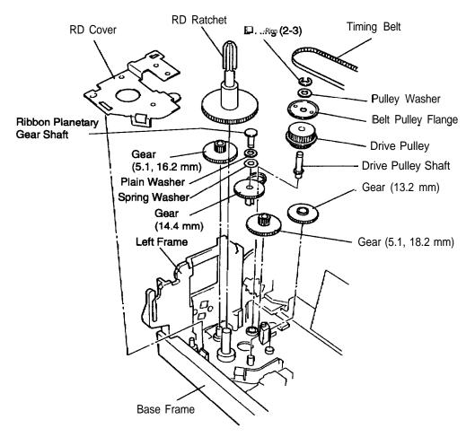
Figure 3-17. Removing the Ribbon Drive Gear Assembly
