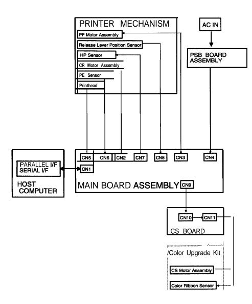
Figure A-1. Cable Connections
