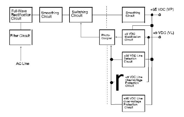
Figure 2-11. Power Supply Circuit Block Diagram
