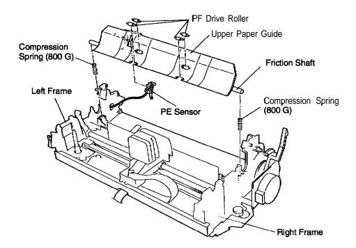
Figure 3-12. Removing the PE Sensor
