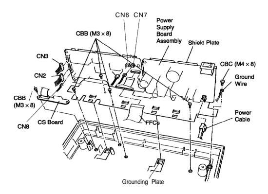
Figure 3-5. Removing the Shield Plate
