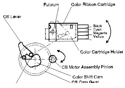
Figure 2-9. Color Shift Mechanism
