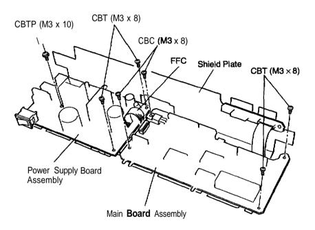
Figure 3-6. Removing the Main Board Assembly and PSB
