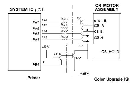
Figure 2-23. CS Motor Assembly Circuit Diagram
