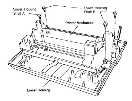
Figure 3-8. Removing the Printer Mechanism
