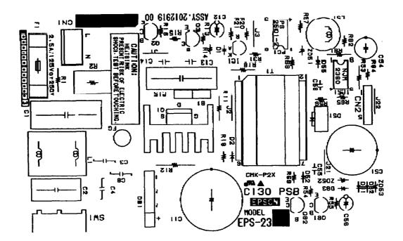
Figure A-5. PSB Board Assembly Component Layout
