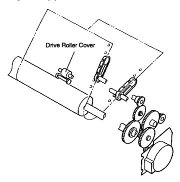
Figure 2-6. Push-Pull Tractor Paper Advance Mechanism
