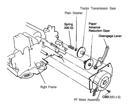
Figure 3-9. Removing the PF Motor Assembly
