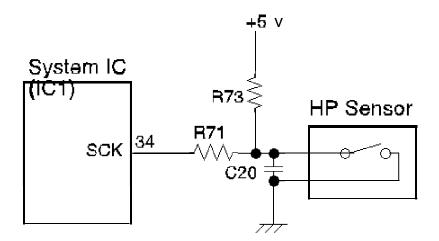
Figure 2-14. Home Position Sensor Circuit Diagram
